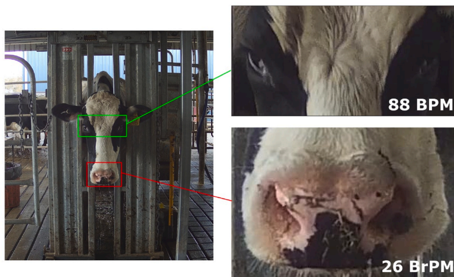
Fig. 1. Example of a video frame from one cow showing the eyes and nose areas identified and cropped to assess heart rate in beats per minute (BPM) and respiration rate in breaths per minute (BrPM), respectively.
